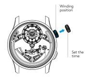
\*The crown should sit flush to the case (position 1) in order to maintain water resistance.
