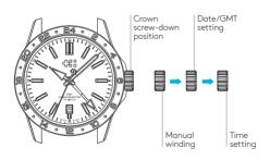
Date correction should not be carried out between 20:00 hrs to 2:00 hrs as the watch gearing will already be aligning itself to change the date.
